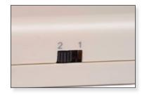
Handset Selector Switch. Selects the correct handset wiring type to suit your telephone.
