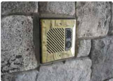
Flush-Mounted 8028 SIP Doorphone using Brass Faceplate
